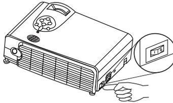
3. Press and hold POWER to start the unit. The back-lit POWER key flashes green and stays green when the power is turned on.
