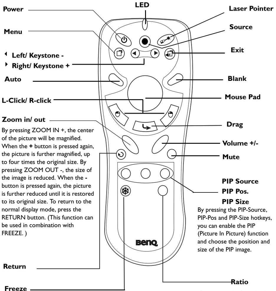
By pressing ZOOM IN +, the center of the picture will be magnified. When the + button is pressed again, the picture is further magnified, up to four times the original size. By pressing ZOOM OUT -, the size of the image is reduced. When the - button is pressed again, the picture is further reduced until it is restored to its original size. To return to the normal display mode, press the RETURN button. (This function can be used in combination with FREEZE.)
