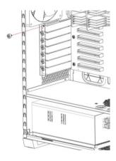
**Step 2** – Remove the slot bracket cover.
