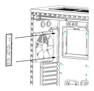
**Step 3** – Line up the motherboard with the I/O shield and the mounting holes, and use the screws provided to secure the motherboard into the case.
