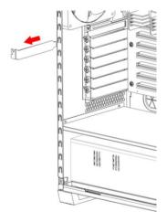
**Step 3** – Install the card, and secure with thumbscrew from step 2.
