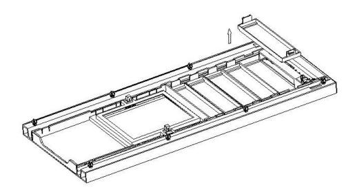
**Step 2** – Decide which bay you will use and remove the corresponding front drive bay cover from the front panel.
