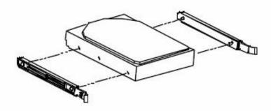
**Step 3 -** Once the drive rails are installed on the drive, slide it into the bay until it clicks in place and is secure.
