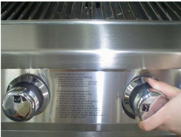
2. Push and turn the main, rotisserie or sear burner control knobs to the "HI" setting. Push the control knob until the burner ignites. The burner should ignite within 4 seconds (if burner does not ignite follow match lighting instructions on Page20). After the burner is lit, adjust the heat level as desired.
