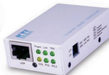
KT-10F supports full/half duplex transmission via its duplex type selector.
