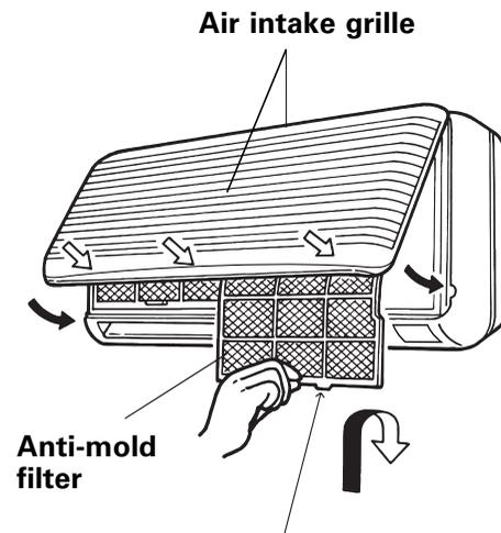
Insert into the groove on the unit.
