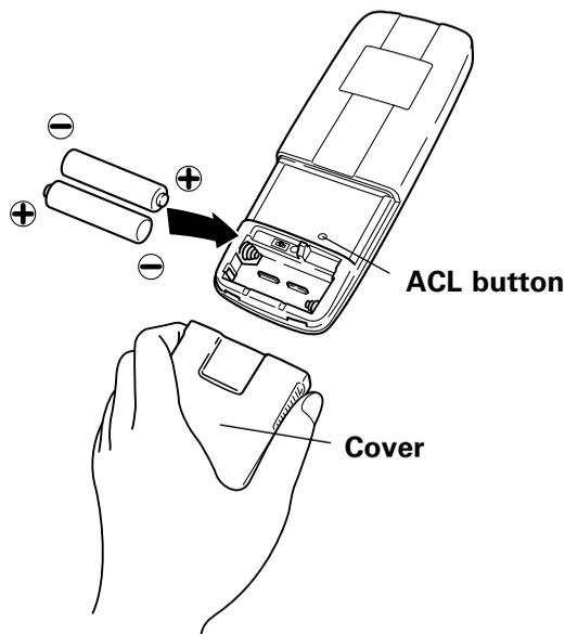
1. Slide the cover in the direction indicated by the arrow and remove it.
