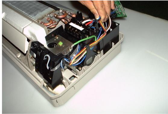
③ Remove the screws (3) attaching the electrical component box, and remove the box from the frame by pressing the tabs at the back of the box.
