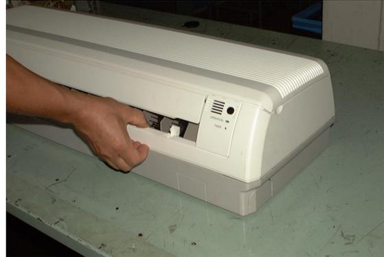
③ Detach the attachment tabs (2) at the top of the grille by lifting the grille.
