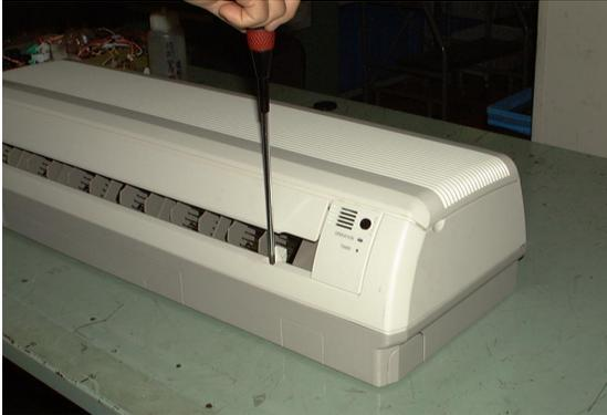
② Remove the fixing tabs (3) at the bottom of decorative grille.
