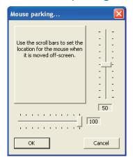
Mouse parking allows you to optionally determine where the mouse pointer for each system should be placed when the focus moves to a different system/ video screen. The **Configure** > **Mouse parking...** option displays vertical and horizontal scroll bars. Use the scroll bars to pinpoint the position that should be used to park the dormant mouse on each screen.
