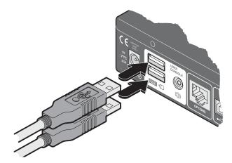
Figure 3-1. Connecting the keyboard/mouse to the user console.
