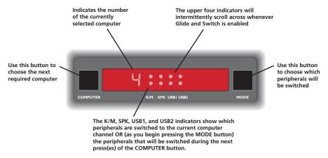
Figure 5-1. Front panel buttons and indicators.
