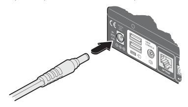
Figure 3-5. Attaching the power adapter lead to the power input socket.
