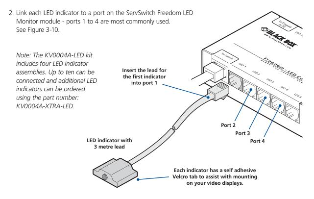
Figure 3-10. Linking LED indicators to the ServSwitch Freedom LED Monitor module.
