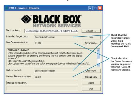
Figure 4-10. KVM Firmware Uploader utility screen with upgrade file selected.
