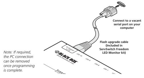
Figure 3-11. Linking the ServSwitch Freedom LED Monitor module to the serial port of a computer.
