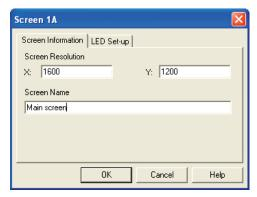
Figure 4-3. Defining the resolution of a screen and (optionally) a name
