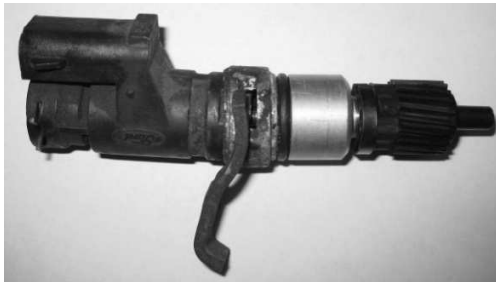
Original speed sensor removed from transmission
