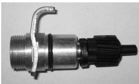
Gear installed on new Ford adaptor
