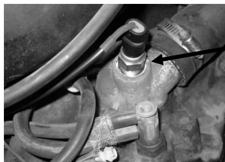
Sensor installed in coolant housing
