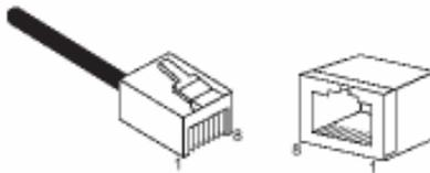
Use unshielded twisted-pair (UTP) or shielded twisted-pair (STP) cable for RJ-45 connections: 100-ohm Category 3 or better cable for 10 Mbps connections or 100-ohm Category 5 or better cable for 100 Mbps connections. Also be sure that the length of any twisted-pair connection does not exceed 100 meters (328 feet).
