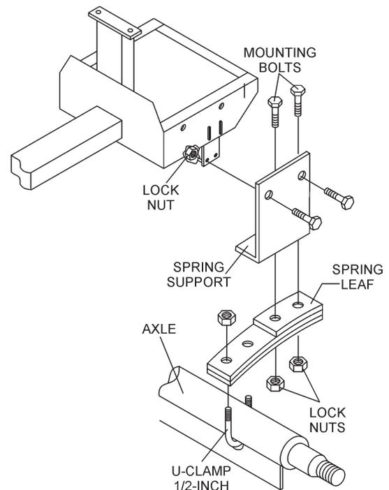
Figure 30. Suspension Components
