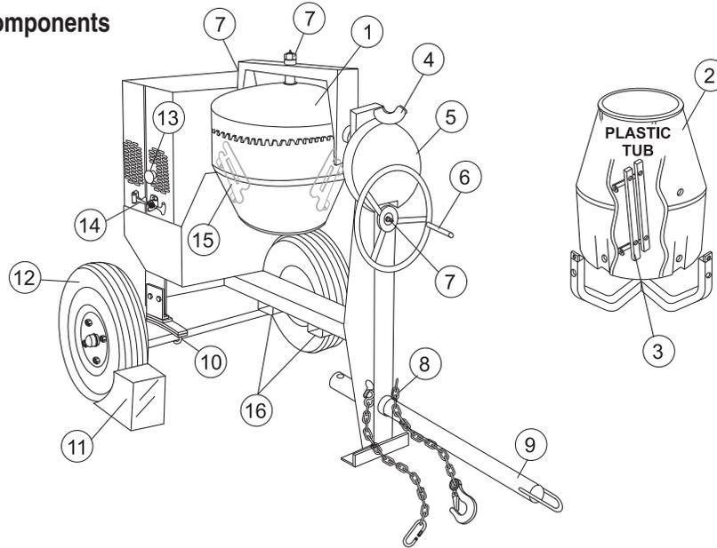
1. **Steel Mixing Drum** — The Multiquip MC94S uses a 6 cu. ft **steel** mixing drum. This drum is to be used for mixing of concrete. Always clean the drum after each use. **DO NOT** use this mixing drum for the mixing of **volatile liquids**.
