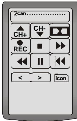
6. Press any of the buttons shown to replace the text “Scan” with an icon. Press < or > to scroll between the pages and display more icons.
