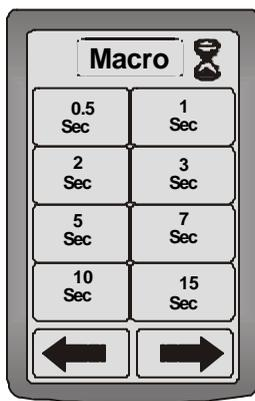
Press one of the listed durations (0.5 seconds to 15 seconds) if you want to have a time delay occur between device commands.
