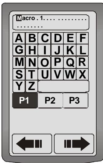
4. Enter the alphanumeric characters from the LCD screen. Press P1 to access upper case letters, press P2 to access lower case letters, and press P3 to access numbers and special characters.
