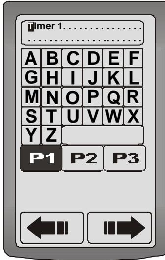
2. Enter the alphanumeric characters from the LCD screen. Press P1 to access upper case letters, press P2 to access lower case letters, and press P3 to access numbers and special characters.
