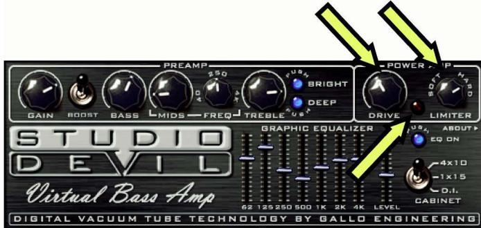
The POWER AMP / LIMITER controls allow you to add compression and loudness to your sound while minimizing the amount of harsh distortion and audible clipping, just like when you turn up the volume on a real amp. Here's how the controls work:
