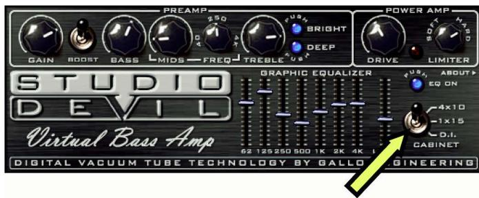
Without a bass speaker cabinet, bass distortion and compression might sound thin and harsh. The “cabinet” switch allows you to select a basic cabinet modeling filter to get the effect of hooking your amp up to a real bass cabinet. There are 3 settings to choose from:
