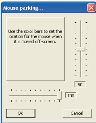
Mouse parking allows you to optionally determine where the mouse pointer for each system should be placed when the focus moves to a different system/video screen. The **Configure > Mouse parking...** option displays vertical and horizontal scroll bars. Use the scroll bars to pinpoint the position that should be used to park the dormant mouse on each screen.
