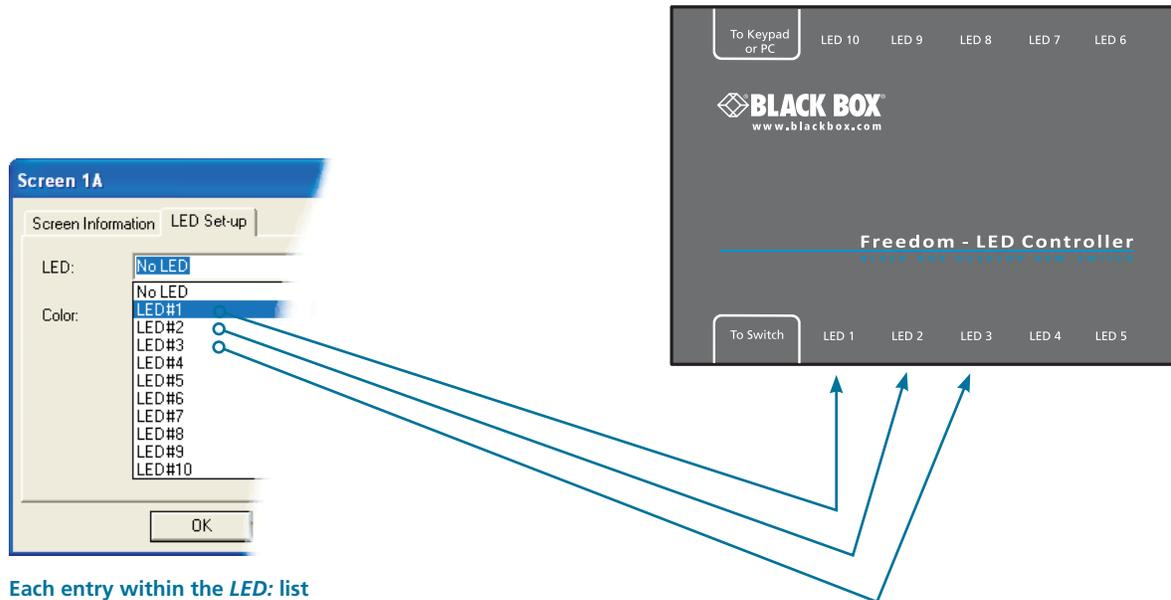
Each entry within the **LED:** list relates to one of the ten output sockets on the ServSwitch Freedom LED Monitor module.
