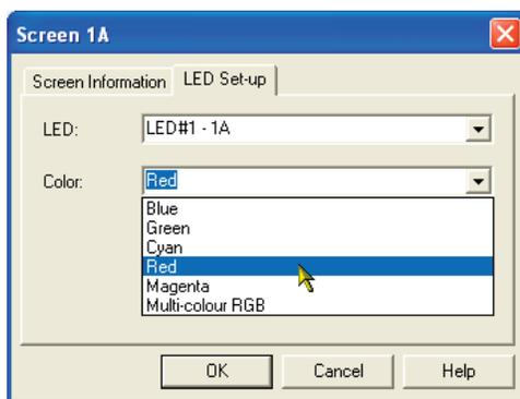
*Note: Each LED indicator can only have one color, so if you associate an indicator with more than one screen and then change the color on a later screen assignment, it will be changed for all the screens in the list for that LED indicator.*
