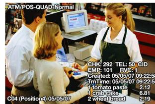
Software provides complete record of customer, cashier and merchandise purchased with text overlaid on video. POS/ATM data is stored on Surveillix DVR for access and search using several criteria. Below is a list of POS devices that are supported by Surveillix POS software. Please regularly check for the most current list by visiting [www.toshibasecurity.com](http://www.toshibasecurity.com).
