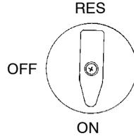
**NOTE:** There's about a 7 to 10 mile (11.2 to 16 km) range on reserve gas. Always refill the gas tank as soon as possible after using the reserve supply.
