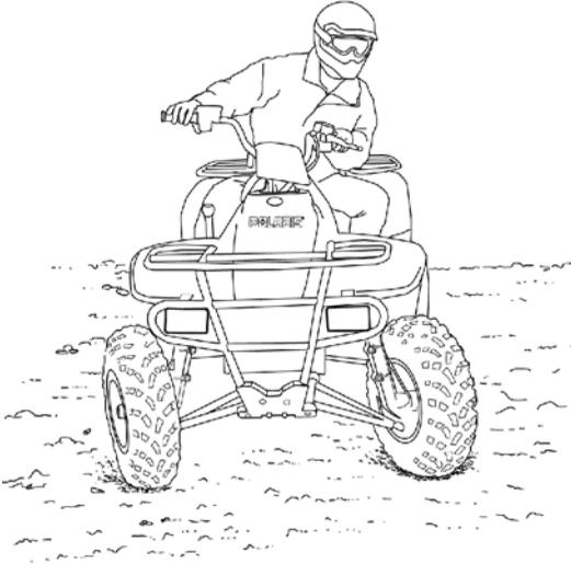
Your Polaris ATV is equipped with a solid rear axle that drives both rear wheels equally at all times. This means that the wheel on the outside of the turn must travel a greater distance than the inside wheel when turning and the inside tire must slip traction slightly.
