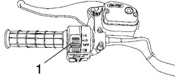
**NOTE:** The lights won't work unless the key is in the ON position and the shut-off switch is in the RUN position.
