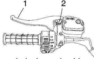
Always test brake lever travel and master cylinder fluid level before riding. When squeezed, the lever should feel firm. Any sponginess would indicate a possible fluid leak or low master cylinder fluid level, which must be corrected before riding. Contact your dealer for proper diagnosis and repairs.
