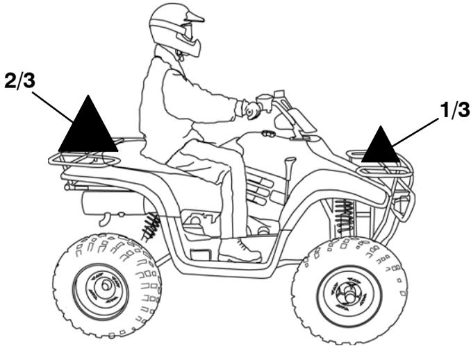
Your ATV has been designed to carry or tow a certain amount of load. Always read and understand the load distribution warning labels on the vehicle, and never exceed the weight capacities outlined in the specifications section of the owner's manual and on the safety decals.
