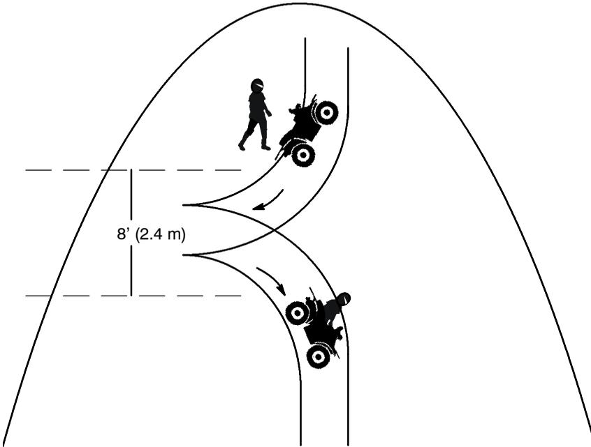
1. Stop and lock the parking brake while keeping body weight uphill.
