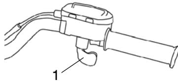
This ATV is equipped with Polaris Electronic Throttle Control (ETC), which is designed to reduce the risk of a frozen or stuck throttle. If the throttle cable should stick in an open position when the operator releases the throttle lever, the engine will stop, and power to the rear wheels will cease.
