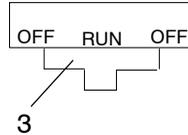
**Main Switch (2) -** To start the engine, slide the stop switch to the center RUN position and turn the main key switch clockwise past the ON position. Release the key when the engine starts.
