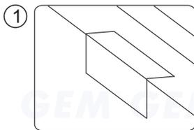
1 Fold the mounting template along the dotted line to a 90-degree angle. Close the door, place the template against the door and frame.
