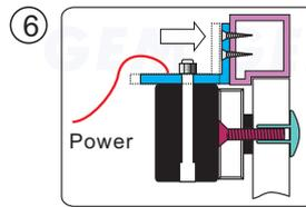
6 Once the position is correct, use the screws to permanently mount the L bracket on the door frame.
