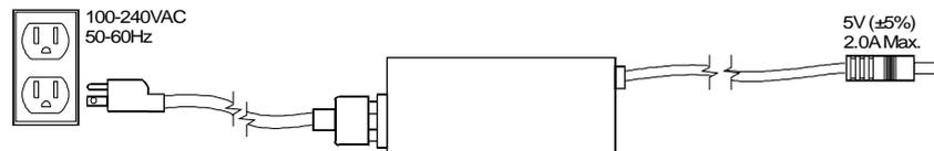
**Figure 3-4. AC/DC Adapter for HP TopTools Remote Control card**
