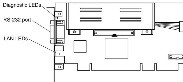
**Figure 3-6. HP TopTools Remote Control PCI Card LEDs**
