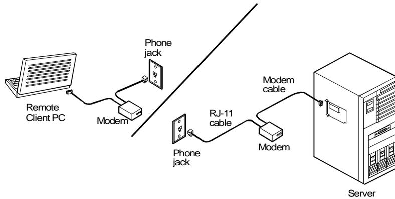
Figure 4-8. Remote Connection Through an External Modem
