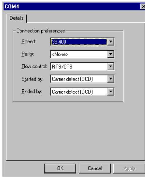
Figure 6-3. Configuring the Server-side COM Port in pcANYWHERE32
