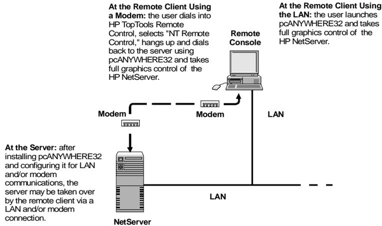
Figure 6-1. NT Console Redirection to a Remote Client
