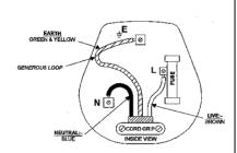
Always ensure that the plug cord grip is fastened correctly.
