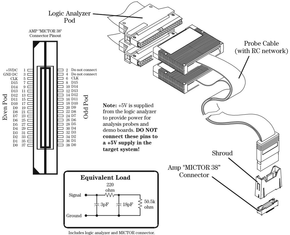
**38-pin Single-ended Probe (E5346A for analyzers with 40-pin pod connectors)**
