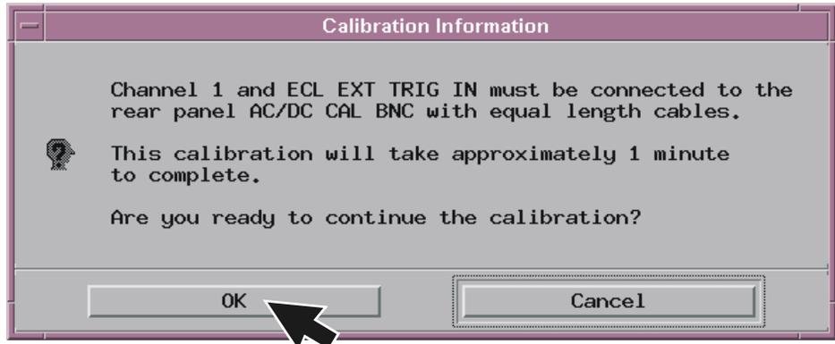
As trigger skew calibration runs, messages appear in the message box on screen. When the Ext Trig Skew calibration is complete, the resulting calibration factors are stored in non-volatile RAM.
