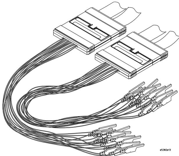
**Soft Touch Probes (E5387A and E5390A for analyzers with 90-pin pod connectors)****Soft Touch Probes (E5387A and E5390A for analyzers with 90-pin pod connectors)****NOTE:**
