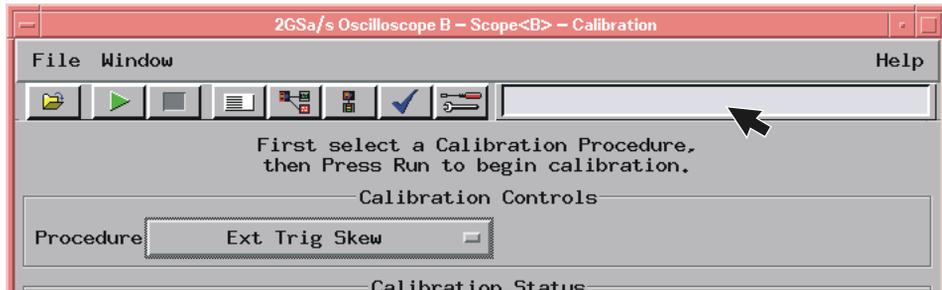
The Calibration Status window indicates pass or fail as each operational accuracy calibration routine is completed. The resulting calibration factors are automatically stored to non-volatile RAM at the conclusion of each calibration routine.
