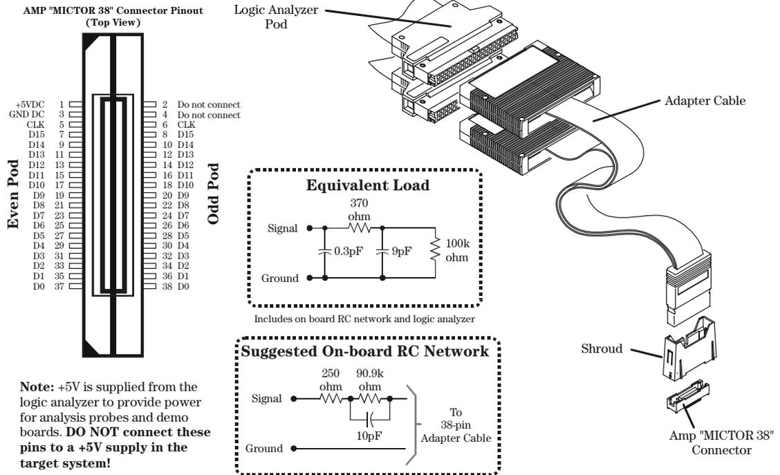
**Note:** +5V is supplied from the logic analyzer to provide power for analysis probes and demo boards. **DO NOT connect these pins to a +5V supply in the target system!**
