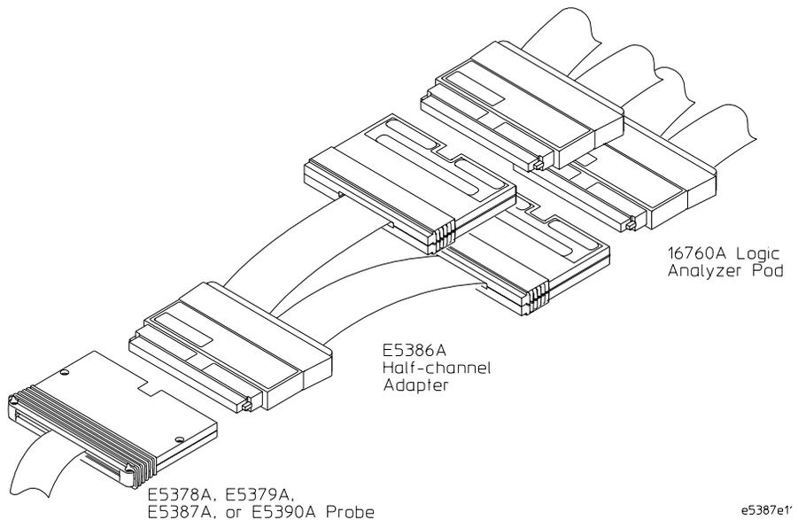
The E5386A Half-channel Adapter has its own ID code. When using the adapter, the logic analyzer recognizes its code rather than that of the probe which is attached to the target. Therefore, the user interface format menu doesn't automatically set thresholds to the right values. You need to go into the threshold menu and select (differential, custom, or standard settings).
