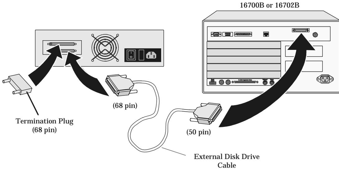
5 Power up the data drive, then the monitor, and then the system (16700B or 16702B).
