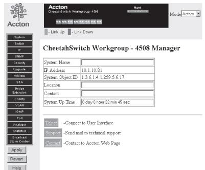
Configurable parameters have a dialog box or a drop-down list. Once a configuration change has been made on a page, be sure to click on the "Apply" button at the bottom of the page to confirm the new setting. Alternatively, you can click on "Revert" to clear any changes prior to pressing "Apply."
