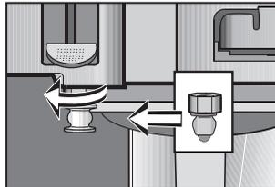
If your machine uses the steam valve nozzle shown in the illustration, replace it with the new nozzle supplied with the cappuccinatore.
