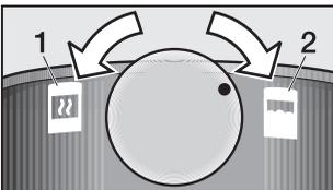
The steam is regulated by turning the valve:
