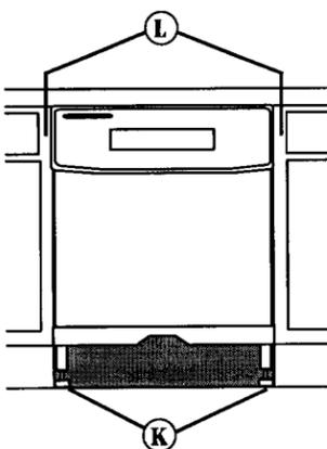
Move dishwasher completely into cabinet opening. Center dishwasher in opening. Check that leveling legs (K) are firmly against the floor. Align the dishwasher door with front of cabinet doors. Check that spacing (L) is the same on both sides.
