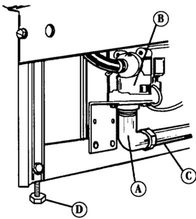
Apply Teflon tape to 90° elbow fitting (A) and connect fitting directly to water inlet valve (B). Attach water supply line (C) to fitting. **Do Not allow the water pipe or tubing to contact the motor or dishwasher legs (D).** Turn on water supply and check for leaks.
