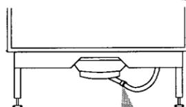
Put the spring-type drain hose clamp (F) over the drain connector (G). Push drain hose (H) onto drain connector. Use pliers to open clamp and slide clamp over drain hose and drain connector. Check that drain hose is securely attached to drain connector.
