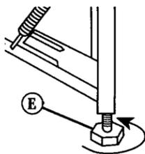
Adjust the front leveling legs (E) the number of turns listed in the chart. The dishwasher should be installed as level as possible from front to back.
