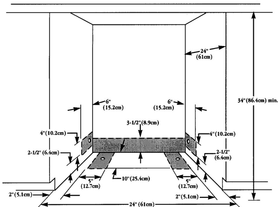
Unshaded area must be free of pipes, wires and drain hose.
