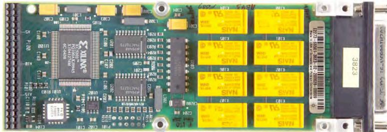
The M221 (formerly Agilent E2273A) provides 8 independent non-latching SPDT switches with maskable interrupts that occur when the requested relay movements have been made. This M Module is useful when high integrity contacts are needed driving microwave relays located in your test adapter.
