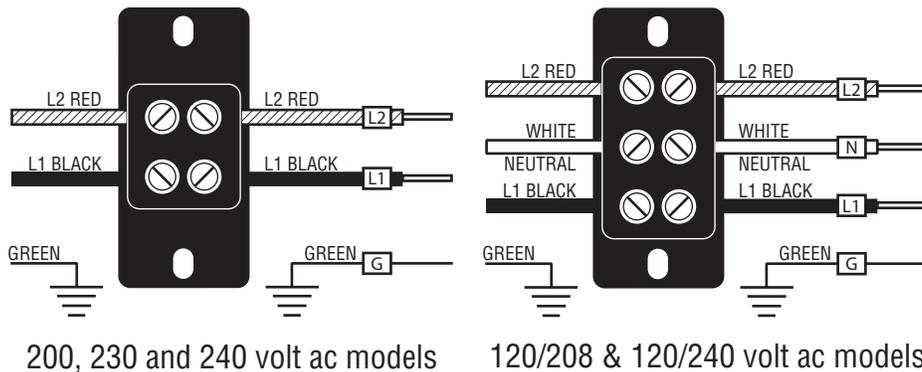
Note: This electrical service consists of 2 current carrying conductors (L1 and L2) and a separate conductor for earth ground.
