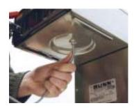
With the sprayhead removed, insert a deliming spring into the sprayhead tube until approximately two inches of the spring remain visible. Saw back and forth five or six times to loosen any lime deposits.
