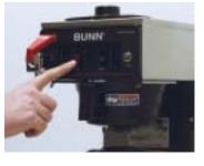
Place the "ON/OFF" switch in the 7. "ON" upper position.
