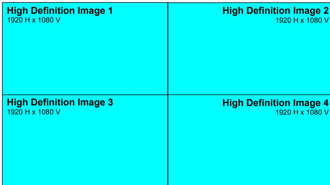
*Sony's 4K SXRD projectors can display four simultaneous HD pictures.*
