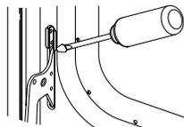
2. Pry door stop clip free and remove from front frame hinge slot. Take care not to scratch finish.
