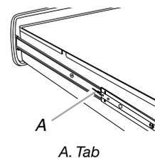
3. Press the tab down on the right side, and lift tab up on the left side at the same time, then pull drawer out another inch.
