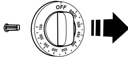
2. Loosen the locking screws inside the oven temperature control knob.
