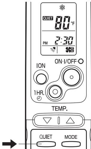
QUIET Mode is used to reduce the fan sound of the indoor unit.
