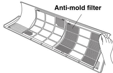
**Cleaning** Use a vacuum cleaner to remove light dust. If there is sticky dust on the filter, wash the filter in lukewarm, soapy water, rinse it in clean water, and dry it.
