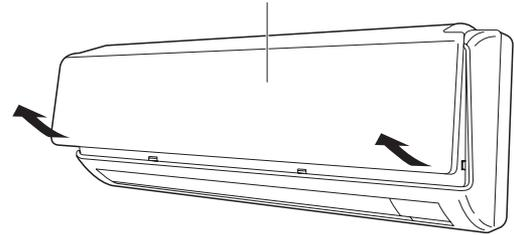
2. Remove the anti-mold filter attached to the rear of the air intake grille.
