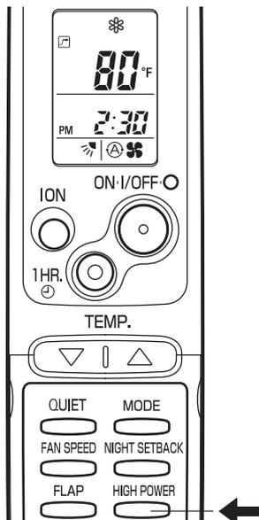
HIGH POWER mode can be used to increase the output of the indoor unit for all operation modes except automatic operation.
