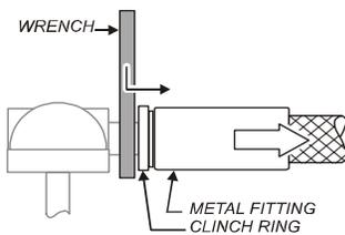
SLIDE WRENCH BETWEEN VALVE AND HOSE FITTING
