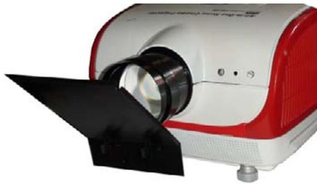
If you use projector in cold day ,you can use the reflected mirror to install on the projector lens(as the above picture),you must adjust the focus lens until the projection image are clearest .
