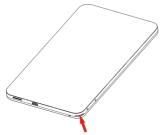
Locate and open the thumb catch on the lower right hand corner (viewed from the back)
