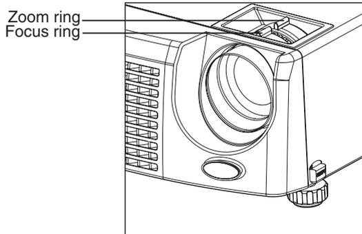
1. Focus the image by rotating the focus ring. A still image is recommended for focusing.
