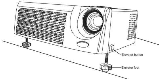
The projector is equipped with an elevator foot to adjust the image height.
