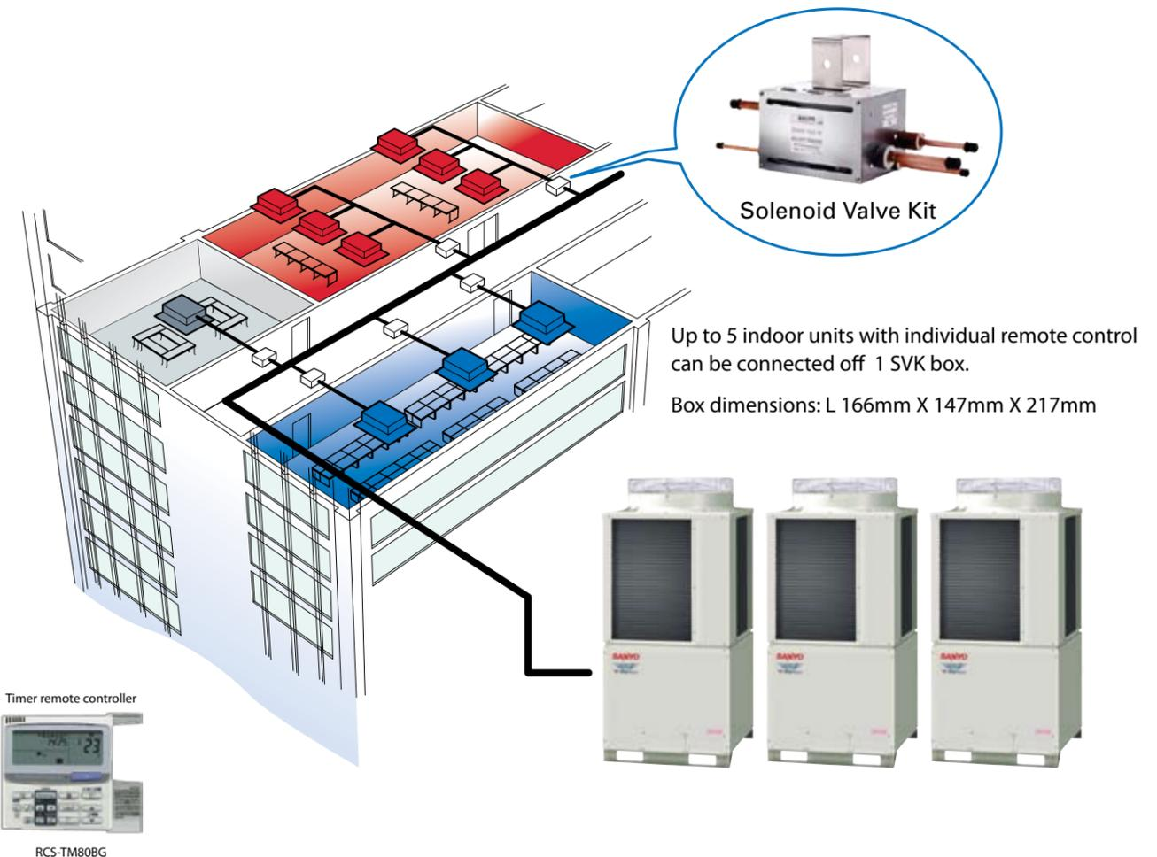
UK Conditions: Cooling Indoor 23°C DB 50% RH Outdoor 30°C Heating Indoor 20°C Outdoor 0°C
