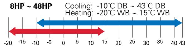
There is improved performance at lower ambient conditions due to SANYO's unique wrap-around outdoor unit coil design and active defrost management.
