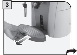
3 Remove the drip tray and wash it under running water.
