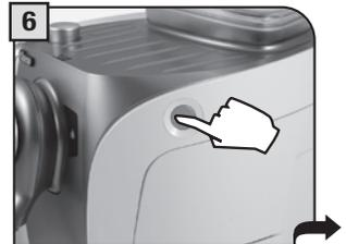
**6** Firmly push down the power button to turn on the machine. The machine performs a self-test.
