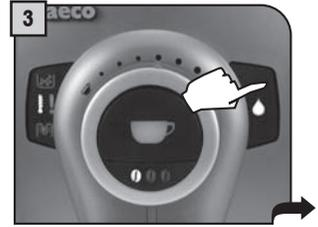
Press the button to select the hot water function. The hot water light will turn on.
