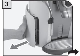
**3** Remove the water tank. We recommend installing the "Aqua Prima" water filter (see page 8).
