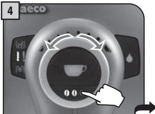
4 Adjust the quantity of coffee by turning the knob. Select the aroma by pushing the button one or more times (see page 10).
