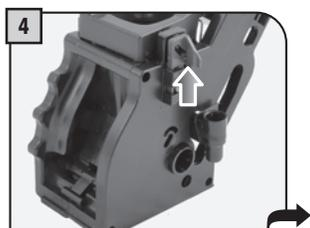
4 Make sure the components are in the correct position. The hook shown must be in the correct position; to check its position, firmly press the "PUSH" button.
