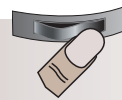
Switch off (machine blocks for 10 min and is ready to be transported)
