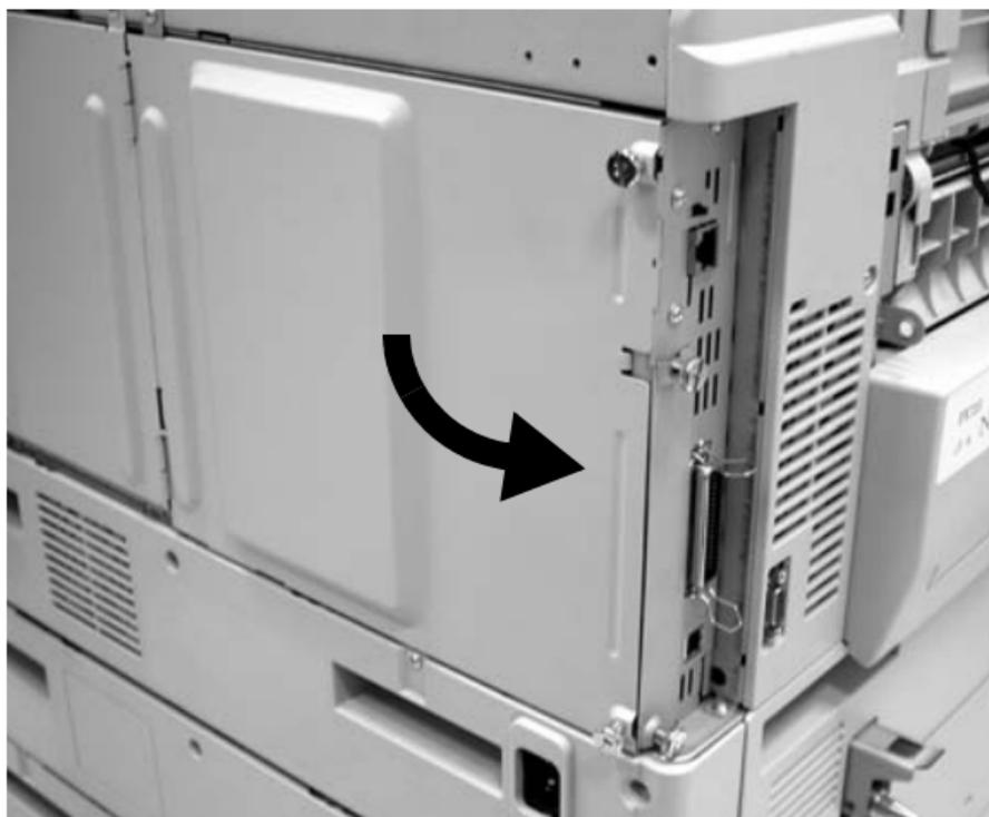
2. Reattach the interface cable, then the power cord.
