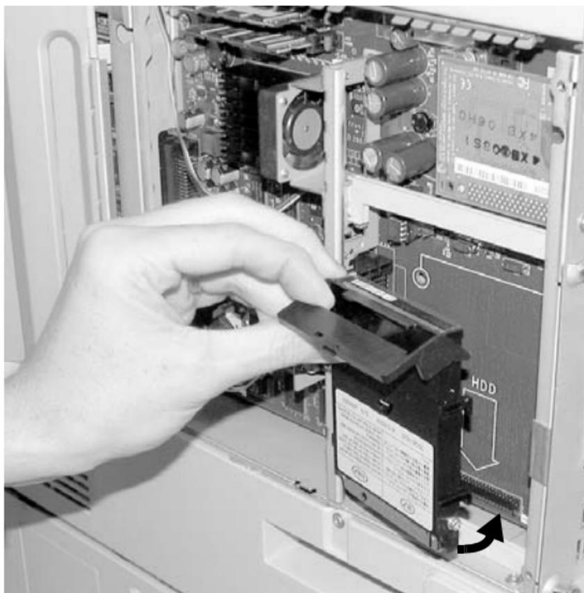
4. Press down on the handle to lock it in place.
