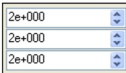
**Figure 2-11.** Numeric Edit Array control
