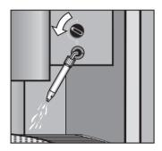
Direct the steam nozzle towards the drip tray and **slowly** turn the steam selector counterclockwise.
