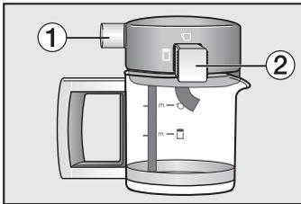
The cappuccinatore has a valve, ①, over the handle and a spout on its side, ②.
