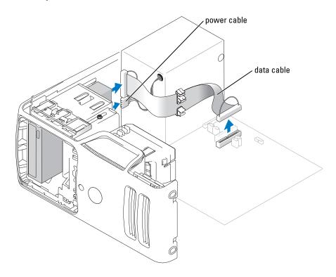
5 Slide the drive latch release toward the bottom of the computer and, without releasing the drive latch release, slide the CD/DVD drive out through the front of the computer.
