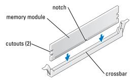
**NOTICE:** To avoid damage to the memory module, press the module straight down into the connector while you apply equal force to each end of the module.
