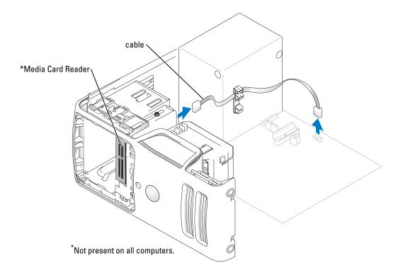
**5** Disconnect the FlexBay USB cable on the back of the Media Card Reader from the Media Card Reader connector on the system board (see page 61) and route the cable through the cable routing clip.
