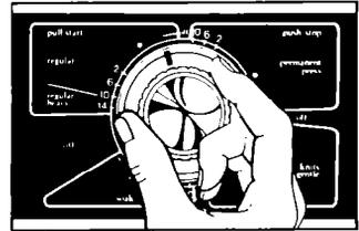
3. Set the washer for a DRAIN and SPIN (see page 10). Let it run for about 30 seconds to mix the antifreeze and water.
