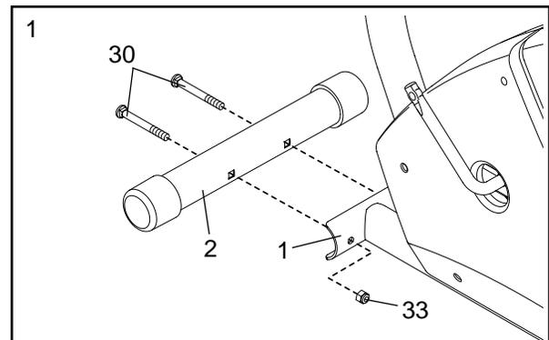
2. While another person lifts the rear of the Frame (1) slightly, attach a Stabilizer (2) with two M10 x 65mm Carriage Bolts (30) and two M10 Nylon Locknuts (33).
