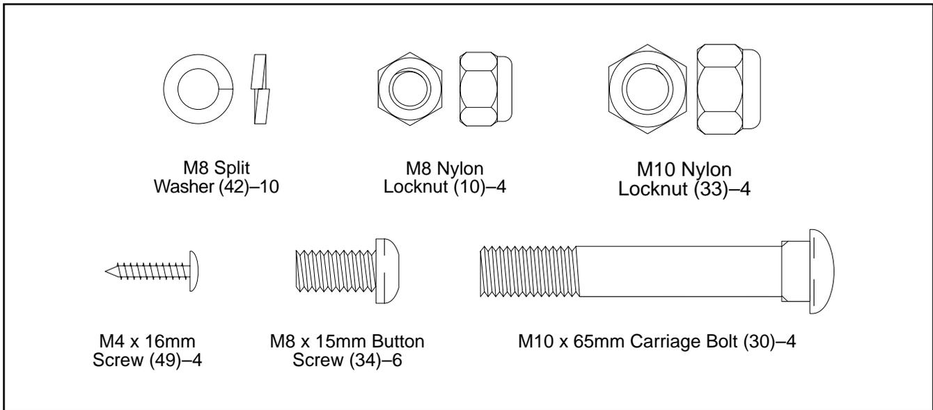
1. While another person lifts the front of the Frame (1) slightly, attach a Stabilizer (2) with two M10 x 65mm Carriage Bolts (30) and two M10 Nylon Locknuts (33).
