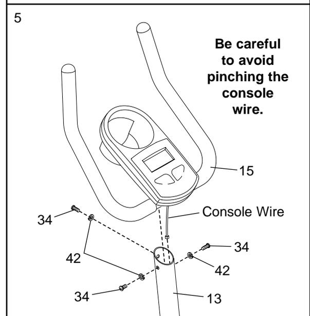
6. While another person holds the Upright (13) in the position shown, connect the console wire to the Reed Switch Wire (43). Next, connect the Resistance Cable (19) to the Lower Cable (45) in the following way:
