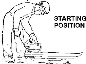
**WARNING:** When starting engine, hold the unit as illustrated. Do not set unit on any surface except a clean, hard area when starting engine or while engine is running. Debris such as gravel, sand, dust, grass, etc. could be picked up by the air intake and
