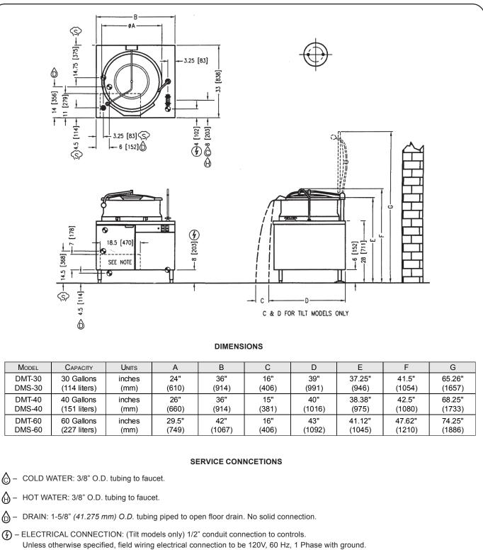
STEAM SUPPLY: 3/4" (19 mm) IPS for incoming steam. MIN 5PSI (34kPa), MAX 35 PSI (241 kPa). Important: Pressure reducing valve required if incoming steam pressure exceeds the kettle rating.
