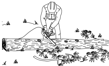
Figure 16 - Bucking Log With Entire Length On Ground
