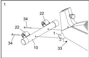
While another person lifts the back of the Frame (1), attach the Rear Stabilizer (9) to the Frame with two M10 x 75mm Carriage Bolts (34) and two M10 Nylon Locknuts (33).
