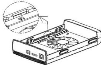
4. Replace the top cover by inserting the tabs into the slots on the bottom of the case.
