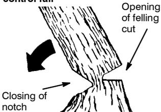
**NOTE:** Before felling cut is complete, use wedges to open the cut if necessary to control the direction of fall. To avoid kickback and chain damage, use wood or plastic wedges, but never steel or iron wedges.
