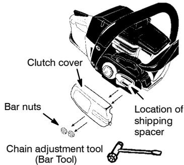
3. An adjusting pin and screw is used to adjust the tension of the chain. It is very important when assembling the bar, that the pin located on the adjusting screw aligns into a hole in the bar. Turning the screw will
