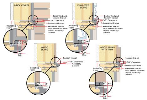
A. **Insert backer rod** into the space around the window approximately 3/8" deep. This should provide at least a 3/8" clearance between the backer rod and the exterior face of the window.
