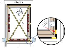
F. Check the interior reveal. Make sure the measurement from the interior face of the window to the interior face of the wall is equal at several points around the window.
