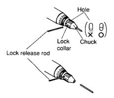
(To prevent accidental operation, remove the battery pack before trying to remove the bit.)
